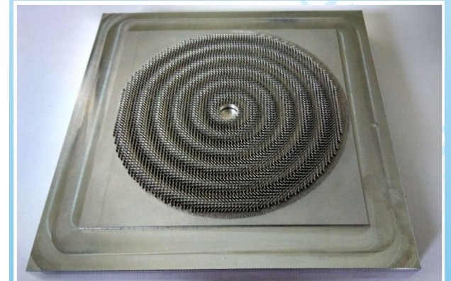
Additively Manufactured Metal only RHCP Ka band Metasurface antenna
