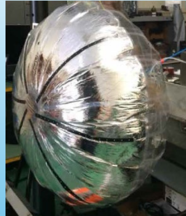
Inflatable X-band antenna prototype for CubeSats
