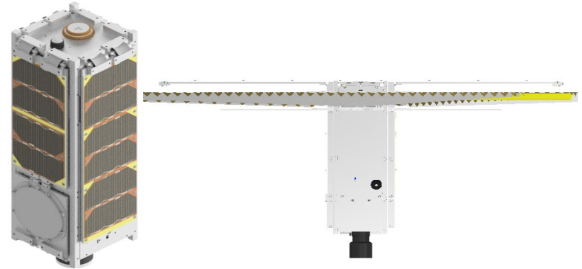
< Initial Design of 3U Cubesat. Stowed(left), Deployed(Right)>
