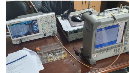
< RF Cable Loss Measurement >
