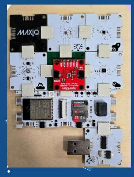
SPC30: Air Quality sensor **KXTJ3:** Accelerometer LTR-390: Measures ambient/UV Light AHT21: Temperature & humidity sensor **Sparkfun BME688:** Gas scanning sensor Extended Core: CPU core **PPU-USB:** for power & programming Spacer: blank chip
