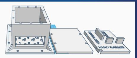
For the main payload housing, we had to include enough room for 4 different circuit boards. We screwed them in both to the housing and to each other. On the top of the payload, we had another level to include a battery pack to power all the boards and multiple hand warmers to keep them running in the cold atmosphere air.
