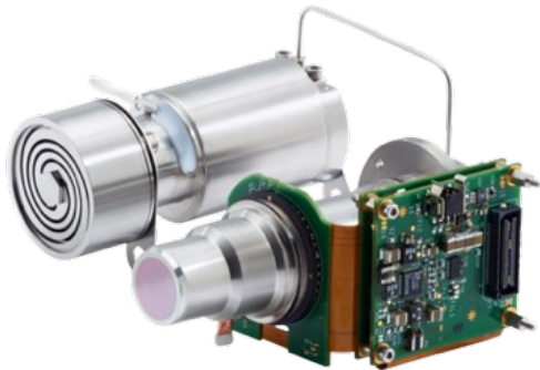
640x512px 12b 120Hz, 80K, Mil-COTS SWIR Imager (Image: AIM)
