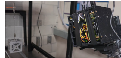
Pictured above is the setup of the CubeSat mounted on the gimbal. Below displays the tracking software (left) and the LIDAR readings (right).
