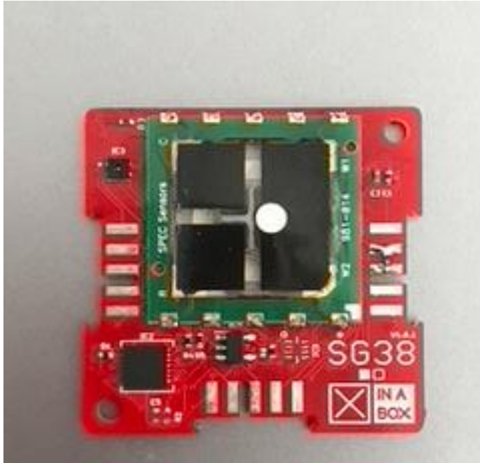
Figure 6 : Student developed \text{SO}_2 sensor
