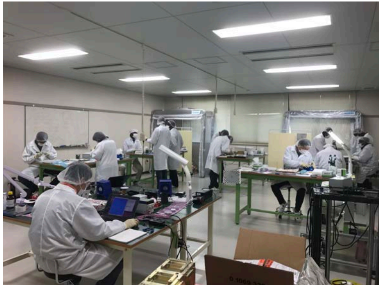
Parallel assembly of 5 satellites (BIRDS-1)
