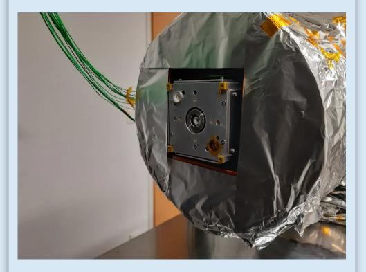
The discrepancies were mainly due to the slight thermal model design differences and the semi-open thermal shroud design in the TVC (as seen on the photo above). The shroud needed an opening for the thruster plumes to be expelled from. As such, the exterior face of the thruster did not see a temperature controlled shroud surface.
