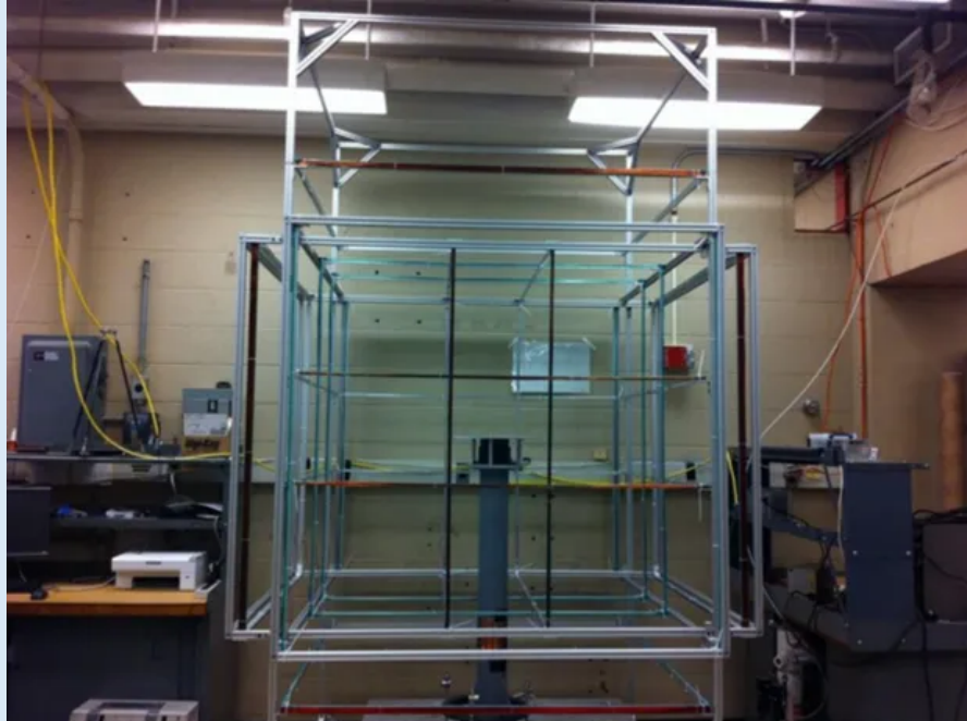
Figure 1: Picture of MIT SSL Helmholtz cage from Prinkey [1]. This cage was used to test our control electronics implementation
