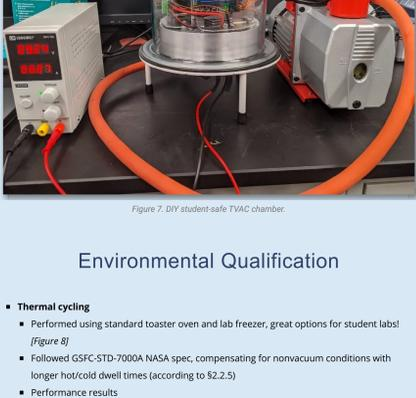
Figure 7. DIY student-safe TVAC chamber.
