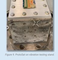
Figure 9. ProtoSat on vibration testing stand.
