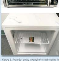
Figure 8. ProtoSat going through thermal cycling in a standard toaster (top) and freezer (bottom).
