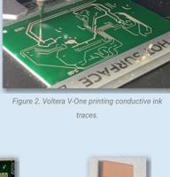
Figure 2. Voltera V-One printing conductive ink traces.
