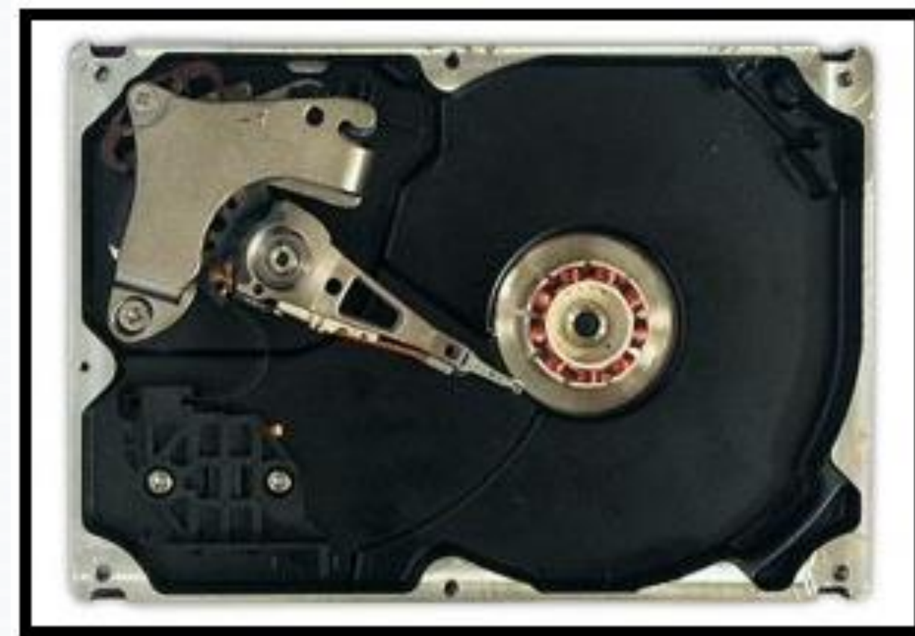
Figure 1: HDD with disks and motor hub removed, exposing copper-colored stator coils surrounding a bearing in the center of the motor.
