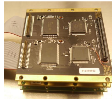
Miniaturized driver electronics to run DM 8 cm x 7 cm x 1 cm
