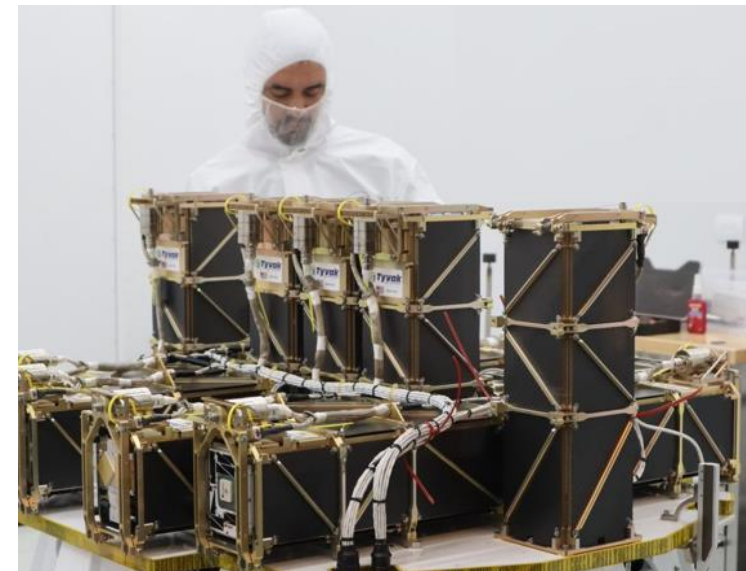
3U RailPODs Readied for flight Photo courtesy of Rocket Lab
