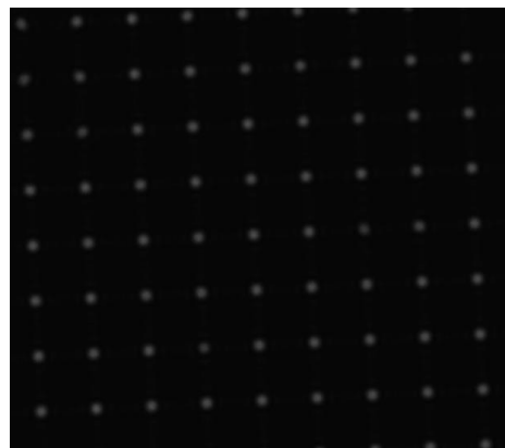
Example spots on Shack Hartmann Wavefront Sensor (spot displacements → wavefront slopes)
