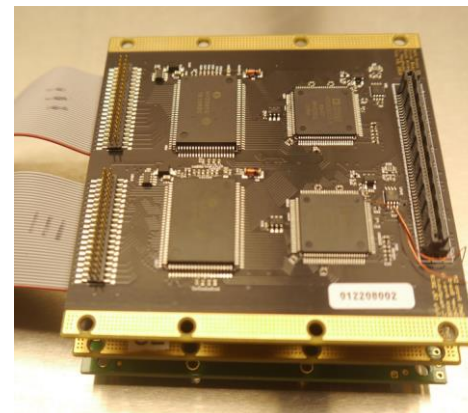
Miniaturized driver electronics to run DM
