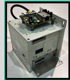
CubeSat SWaP: Radar payload electronics packaged into 1.3U CubeSat form factor
