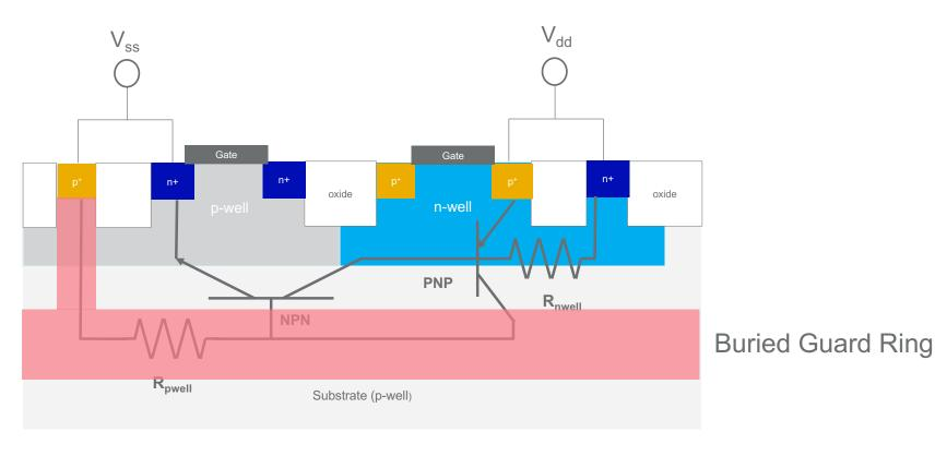
HARDSIL® creates a highly conductive layer underneath the CMOS devices and wells combined with a high conductivity connection to well contacts
