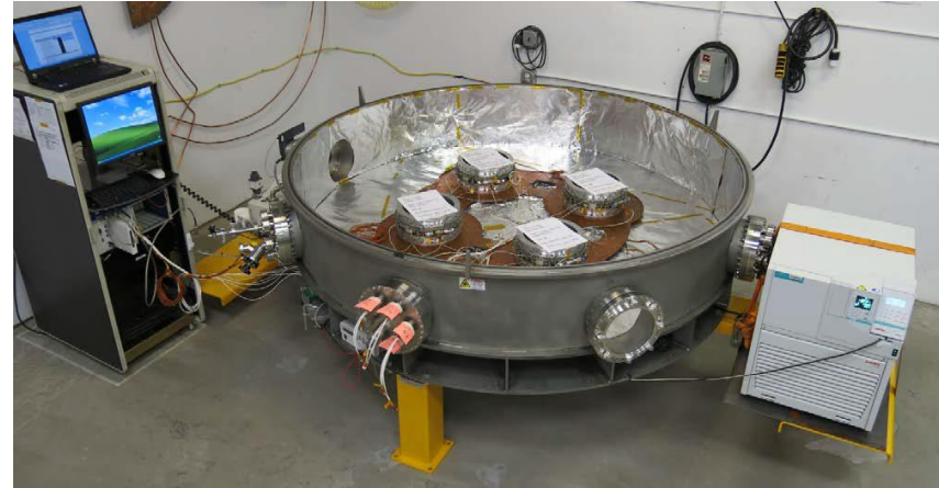
At PSC we can qualification test four test items simultaneously and autonomously in a custom made thermal-vacuum chamber
