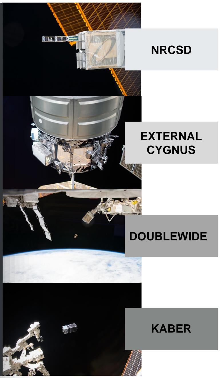
**Over 180 CubeSats deployed** into low-Earth orbit via the NanoRacks CubeSat Deployer on the International Space Station
