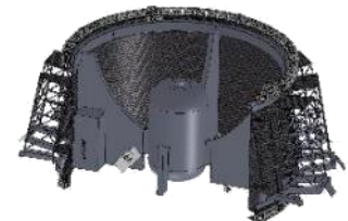
Small Launch Adapter and SL-OMV (Ø38'')
