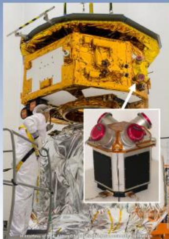
Eight First-Generation Busek Electro Spray Thrusters on LISA Pathfinder (NASA ST-7)
