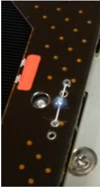
Intact tie-down after vibration testing
