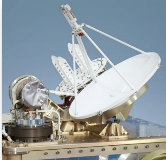
SCaN Testbed Ka-band and S-band Antenna Positioning System (APS)
