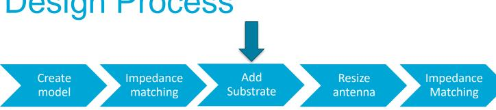
Substrate adds physical support between patch and ground
