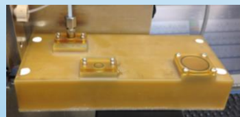
1.5kg-Capacity, Thermoplastic Solid Iodine Storage Tank; 22psi Proof Pressure
