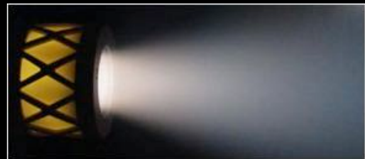
Busek BIT-3 solid I 2 ion propulsion
