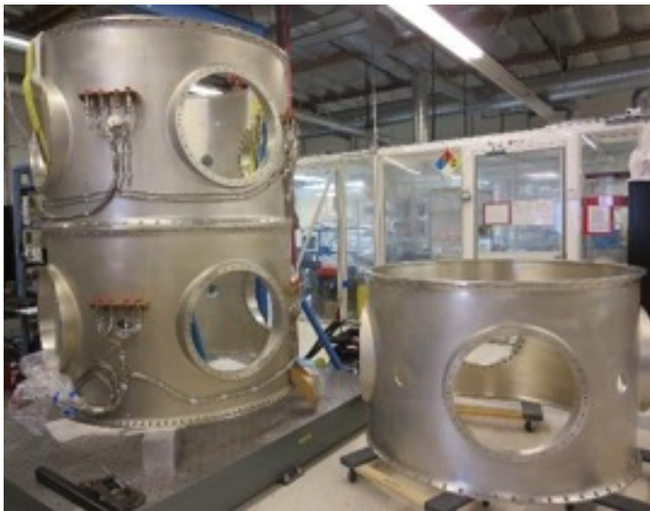
ESPA rings at Moog CSA in Mountain View
