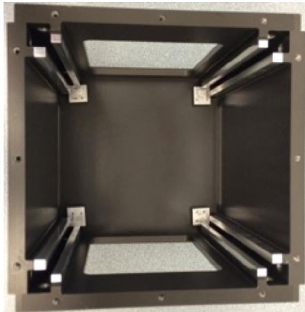
1U Test-POD with soft rails
