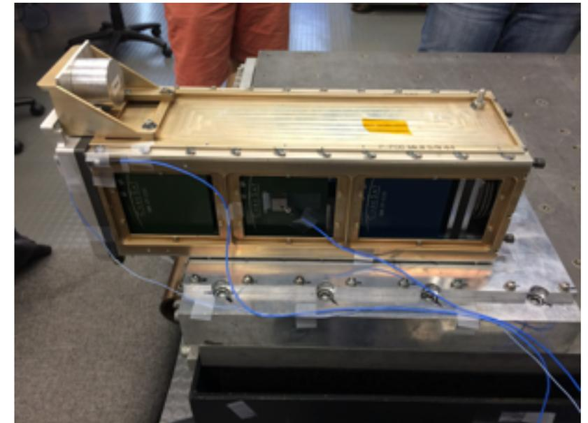
Z-Axis Test Setup with Modified Door
