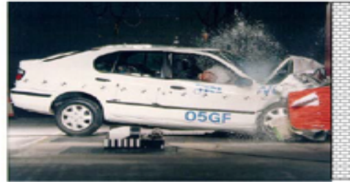
mid-size car of 1.5 tonnes at 50 km/h
