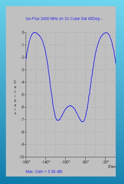
Rectangular plot showing the gain from the far satellite horizon, thru the nadir, and to the near satellite horizon.
