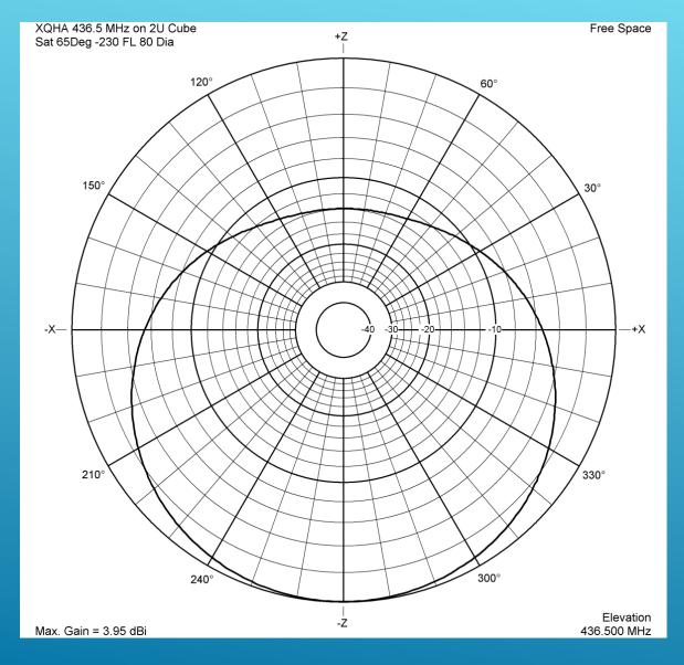
Polar plot showing the gain from the far satellite horizon, thru the nadir, and to the near satellite horizon.
