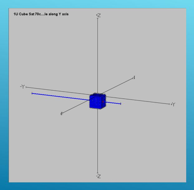
436.5 MHZ HORIZONTAL MONOPOLE ON RIGHT, AND A 145 MHZ MONOPOLE ON LEFT SIDE OF A 1U SMALL SATELLITE
