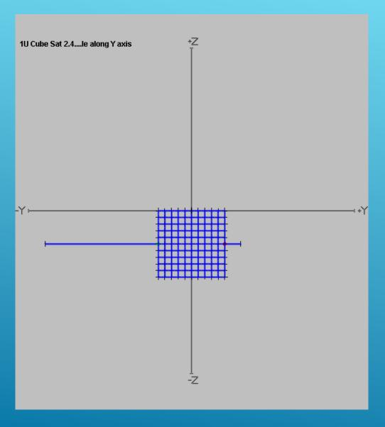
2400 MHZ HORIZONTAL MONOPOLE ON RIGHT, AND A 436 MHZ MONOPOLE ON LEFT SIDE OF A 1U SMALL SATELLITE
