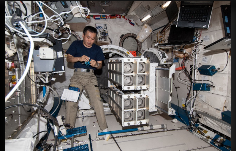
9. ISS Crew un-install first 8 NRCSDs; repeat install/deploy for second set of NRCSDs
