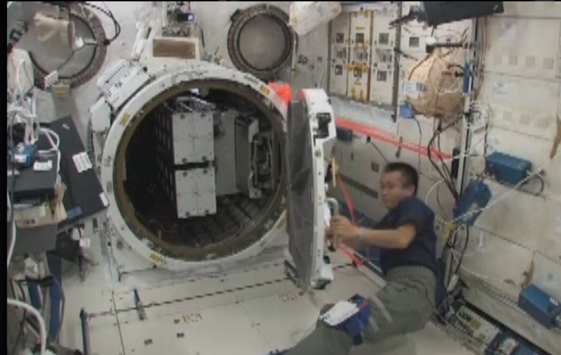
4. JEM Air Lock depress & slide table extension
