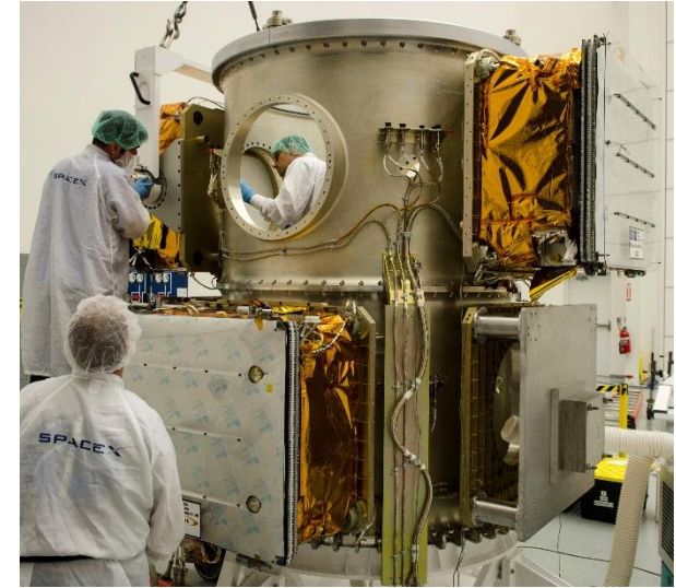
OG2 Constellation of eight spacecraft on two stacked ESPA rings with SoftRide vibration isolation for launch on SpaceX Falcon 9 (Photo credit Sierra Nevada Corporation and ORBCOMM)
