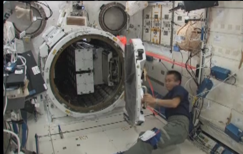
4. JEM Air Lock depress & slide table extension
