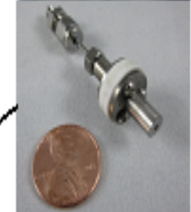
1/16" Subminiature Electride Cathode as Ion Beam Neutralizer; Heaterless, 5W Nominal
