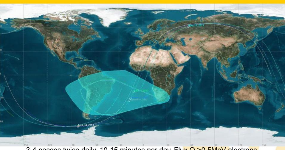
3-4 passes twice daily, 10-15 minutes per day, Flux O >0.5MeV electrons, 23-94 MeV protons 1-10K /cm² sec str, 1990-1996, 2000-2006, CEASE/TSX-5, LET vs Cross-Section curve starts at 2MeV.cm²/mg, probabilistic, must collide
