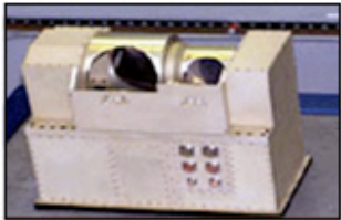
Advanced Technology Microwave Sounder (ATMS)
