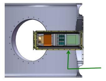
CSD is cantilevered off of Interface Plate
