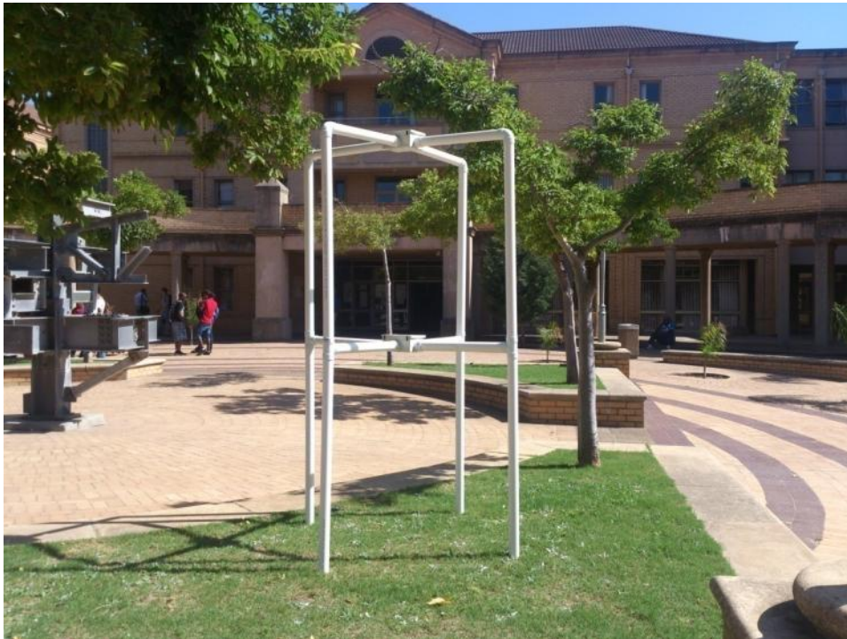
HF Ground Station Antenna Array Constructed at SANSA, Hermanus Designed and developed internally
