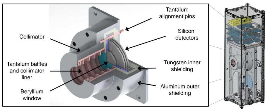
Measures directional differential flux of 9 to 40 MeV protons & 0.5 to >3.3 MeV electrons with 6 sec. time resolution
