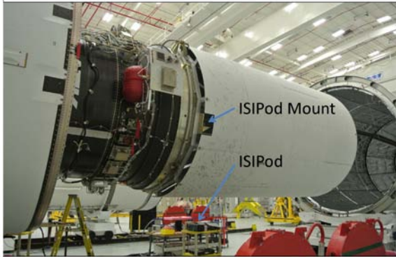
Image of Spaceflight's ISIPod Testing prior to mating to Cygnus Mass Simulator
