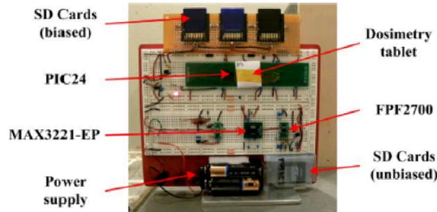
Fig. 1. Test jig used for TID tests
