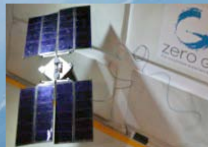
0-g Panel Deployment Testing
