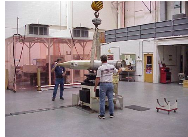
Wallops Moments of Inertia (MOI) and Center of Gravity (CG) determination
