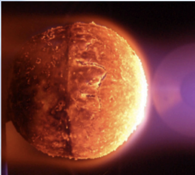
Ablation test in Plasmatron for the YES 2 capsule
