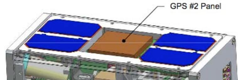
AutoCad drawing of CTECS custom dual patch antenna embedded in the MTV satellite panel.
