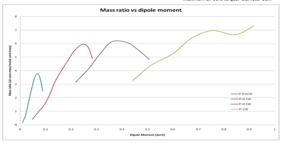
The air core magnetic torquer are convenient in terms of mass only if very low required dipole moment <0.06Am2
