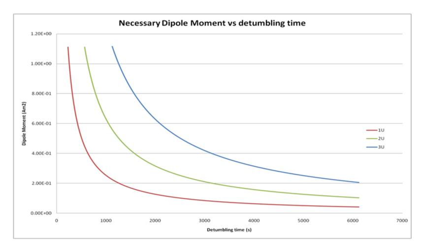
0.2 Am2 Dipole Moment Magnetic Torquer is a good compromise to have perform detumbling in a reasonable time
