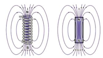
Introducing a metal core in the magnetic torquer increase the dipole moment of the solenoid The metal core is able to increase the dipole moment up to 300 times!
