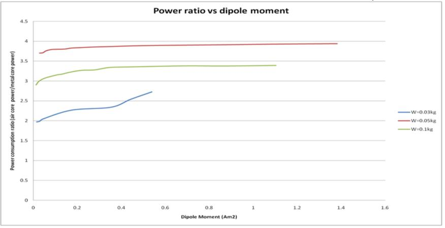
The metal core torquer is always more efficient wrt the air core one for a given Dipole moment and a maximum mass
