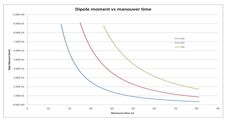
0.2 Am2 Dipole Moment Magnetic Torquer is a good compromise to have good agility for 1U, 2U and 3U cubesat
