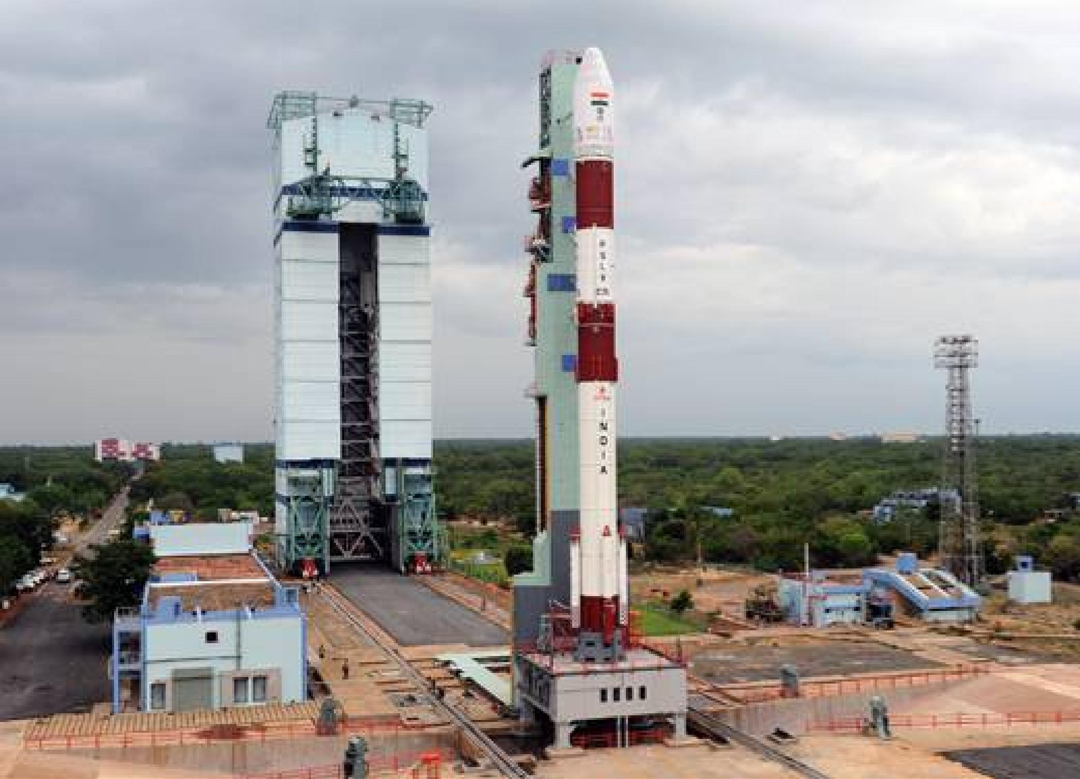
PSLV C-15 after the Mobile Service Tower (MST) has rolled back
