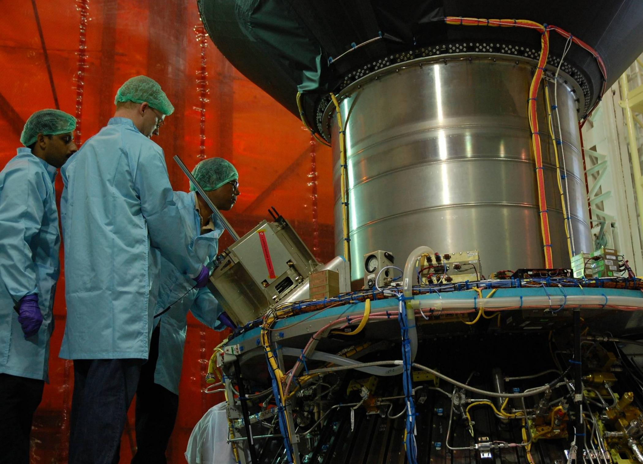
**Mounting of AISSat-1 and its XPOD on the PSLV EB Deck**
