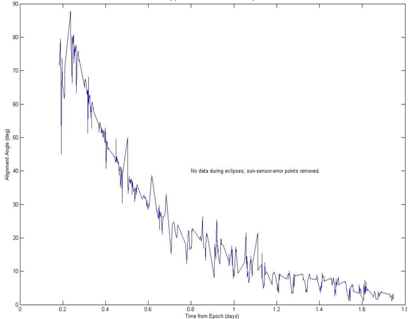
**Momentum align controller reducing angle between spacecraft Y-axis and orbit normal towards 0°**
