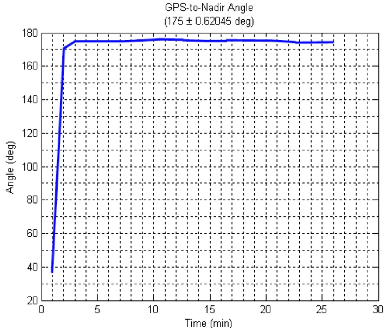
Wheel pitch controller aligning GPS antenna towards zenith
