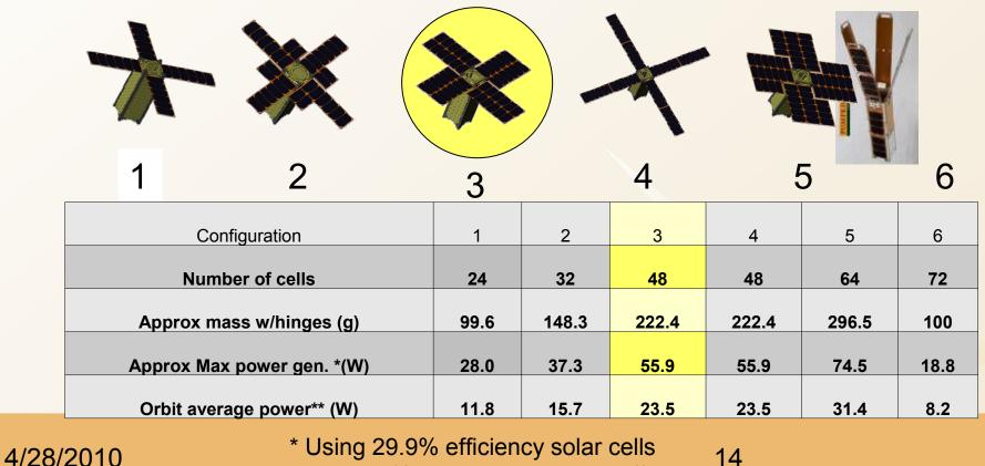
\* Using 29.9% efficiency solar cells
