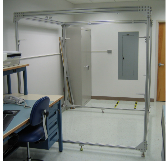
Helmholtz cage under construction
