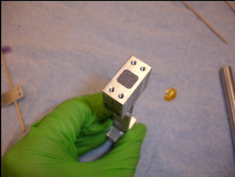
Cantilever beam tip mass shown filled with a fine tungsten powder before being capped off with a lid
