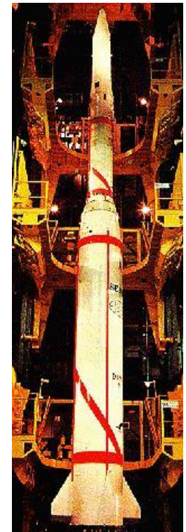
The pressure-fed Diamant A rocket succeeded in placing a satellite into orbit on its first try in November of 1965
